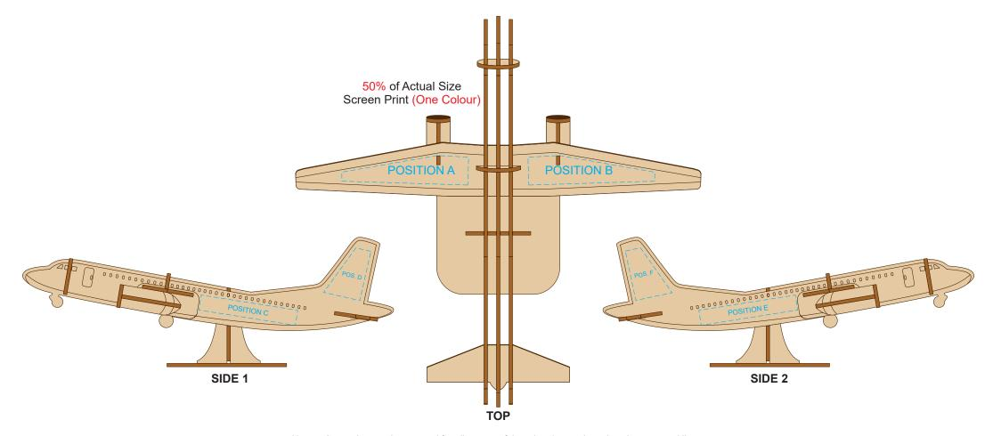
Up to a 2mm tolerance is expected for alignment of the printed artwork against the engraved lines. Slight inconsistencies are to be considered acceptable if the artwork is printed over an engraved line.
